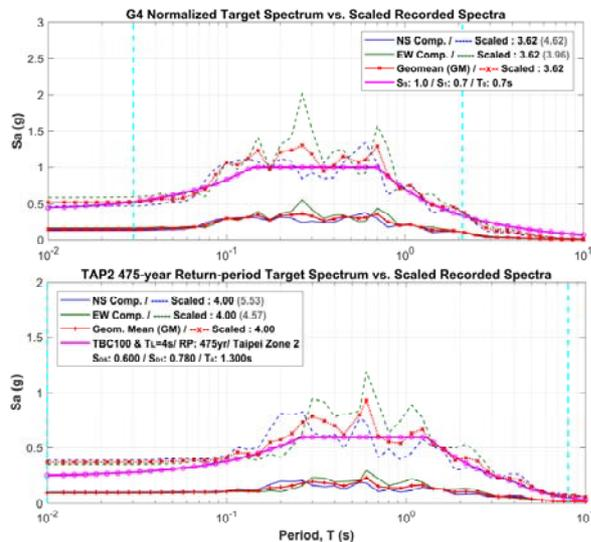
Fig. 4 Scaled and non-scaled recorded spectra of the smallest  $MSE_0$  for group G4 (top plot) and group TAP2 (bottom plot).
