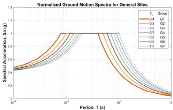
Fig. 1 Seven normalized target design spectra for general sites (EPA of 0.4 g).
