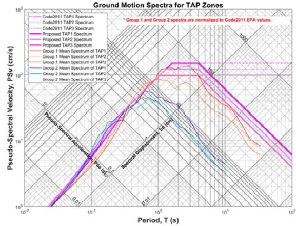
Fig. 2 Three target design spectra for Taipei Basin sites (thick solid lines).
